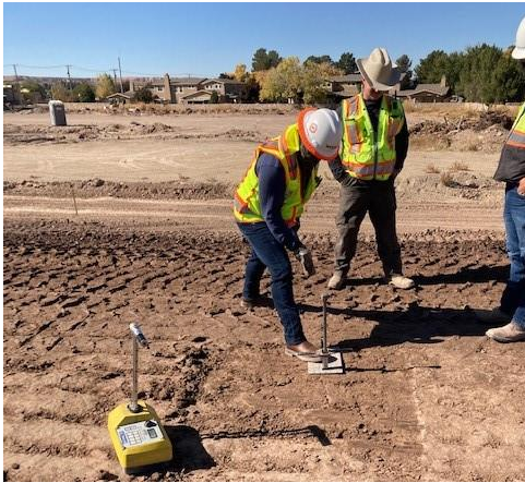
Personnel getting ready to perform test to verify the level of compaction of the western levee. 1/16/2020
