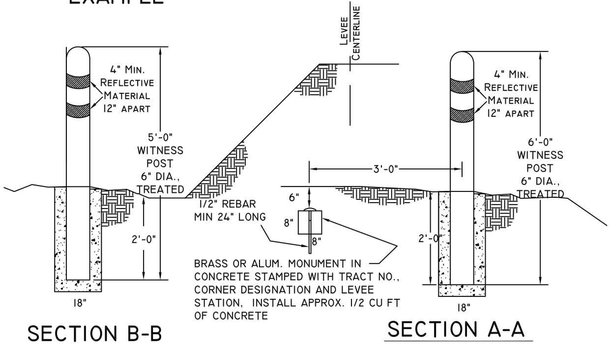
I. WITNESS POST SHALL BE INSTALLED IN AUGERED HOLE;
