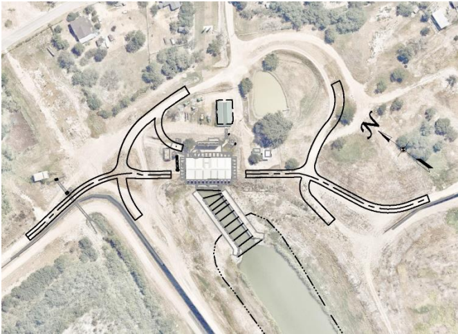
Excerpt from construction drawings showing site layout and location of new levee.
